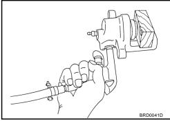
Using a flat-bladed screwdriver, remove piston seals from cylinder body.
