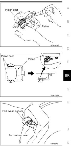
3. Apply brake fluid to piston, and press piston into cylinder body by hand to assemble piston side lip on piston boot properly into groove on piston.
