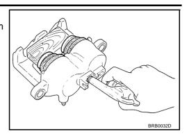
5. Using a flat-bladed screwdriver, remove piston seal from cylinder body.
