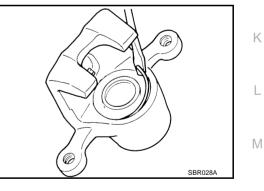
4. Place a wooden block as shown in the figure, and blow air from union bolt mounting hole to remove pistons and piston boots. **CAUTION:**
